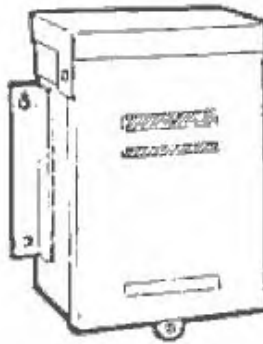
GFI TO INSTALL IN BRANCH CIRCUIT
